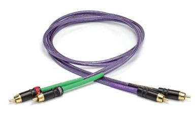
he Purple Flare is a fullyshielded design using six, silver-plated 99.9999% OFC solid-core conductors, precision wound in a minimum cross-section configuration, insulated via FEP, and hand-terminated in the USA.
