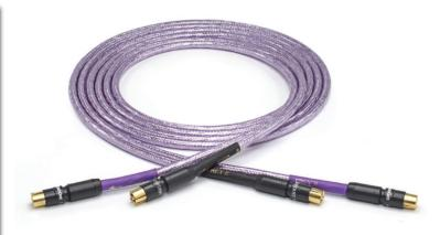
uilt with Nordost's proprietary Micro Mono-Filament construction, to create a virtual air dielectric complete with suspension system, the Frey 2 provides silver-plated OFC solid-core conductors and FEP insulation throughout.
